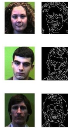
Figure 6: Edge detection (left) Original Image (right) Result of edge detection
