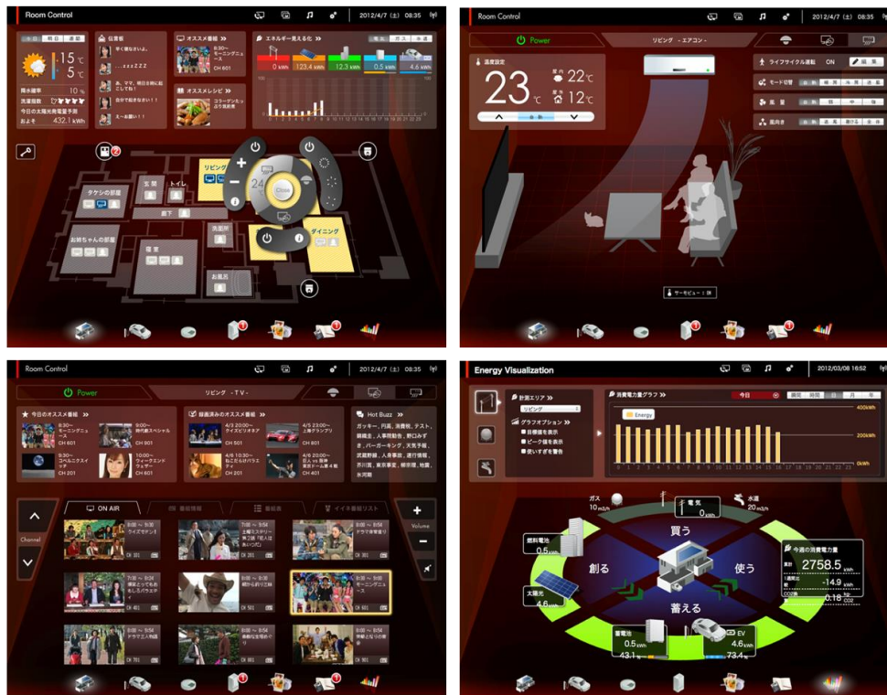
Fig. 10 The screens of the proposed handheld device: (a) Top left: The main screen with current conditions, “command circle,” and icons on the bottom bar. (b) Top right: The screen showing the detailed setting of a room air conditioner. (c) Bottom left: The screen for controlling the television set; the TV programs currently being aired are displayed on this screen. (d) Bottom right: The screen showing the overall energy input/output, storage and consumption.
